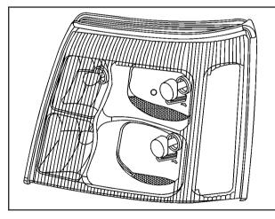
2. Measure the distance from the ground to the aim dot on each low beam lamp. Record this distance.
